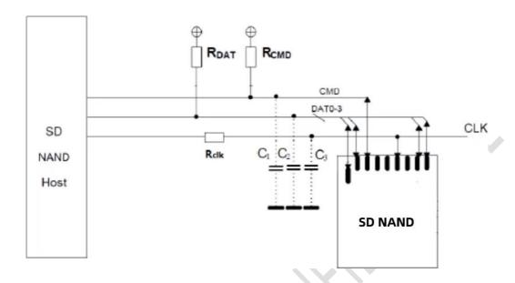
RDAT and RCMD (10K $\sim$ 100 k $\Omega$ ) are pull-up resistors protecting the CMD and the DAT lines against bus floating when Nano SD NAND is in a high-impedance mode.
