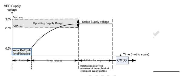
Host needs to keep power line level less than 0.5V and more than 1ms before power ramp up.
